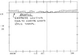
The RTA levels are weighted higher with increasing frequency. This is due to wider bandwidths, more 1 Hz levels being added together. The equivalent narrow band spectrum can be had by subtracting the bandwidth weighting term from each bandwidth level.
