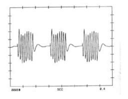
the duty cycle. A ramped attack and decay would reduce the ringing effect. Although the pure tone quality of each burst is degraded by the low level ringing, this coloration provided unique cues for the subjective perception of attack transients. At about 2 dB articulation level, the LF ringing loses audibility—this may suggest a method to evaluate perception thresholds of tonal transients.
