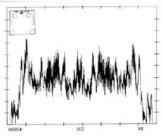
e. Finally we have added the rear wall. A 16x3 + 11x5 center column and 4 sets of  $11x5 \frac{1}{2}$  Rounds with one more pair on the front wall. The result is a very wide and steady articulation pattern that extends even into the deepest bass. Peaks and valleys now even more are soft, rounded. The room still retains a strong, comfortable ambience.
