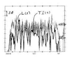
2. This curve is a linear frequency sweep and the mean TI requires log frequency weighting. If a log frequency sweep was used instead of linear, then straight integration of the TI in time would produce the mean TI.
